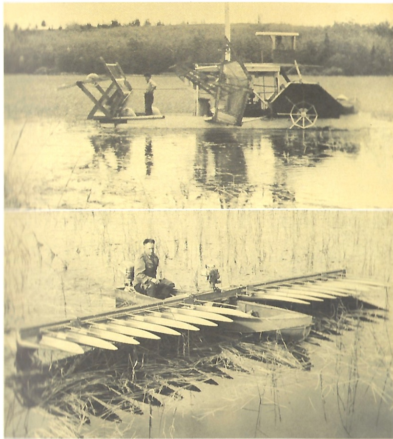
Mechanized harvesting of wild-rice. Upper: The harvester developed by H. B. Williams at Lac du Bois, Man. Rotating flails beat the ripe grains onto a fine-wire screen as the scow, mounted on two slender floats, is propelled through the rice beds. (Photo by National Film Board) Lower: Z. Durand of Winnipeg and the harvester he invented. Tapered aluminum scoops catch the grains and direct them to a long collecting trough mounted across the skiff. Oscillating rods jiggle the wild-rice stems as the craft moves through the beds. (Photo by National Film Board)
