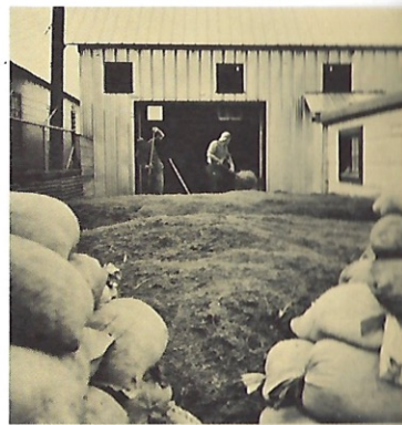
Bags of green rice received at a processing plant in Winnipeg are first emptied onto a long pavement. The grain is then forked over and spread to dry, before it goes to the parching ovens in the shed beyond.
